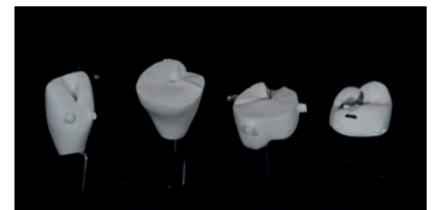
Figure 5: Common milling faults from left to right: chipped screw hole channel caused by fractured burr, complete failure of molar restoration caused by fractured disc, holes within the occlusal surface, restoration designed to minimum thickness followed by inaccurate CNC calculation
